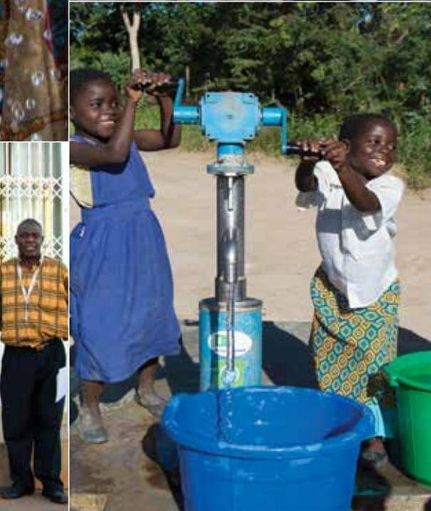
During a year and a half of use in Zolomondo, for instance, the LifePump has shown no signs of degradation or reduction in efficiency. While some pumps can take 30 minutes or more to first get water, the LifePump produces water almost immediately and averages a flow rate of about 2.5 gallons per minute. In Nyirenda's words, "The pump has no mistake."
