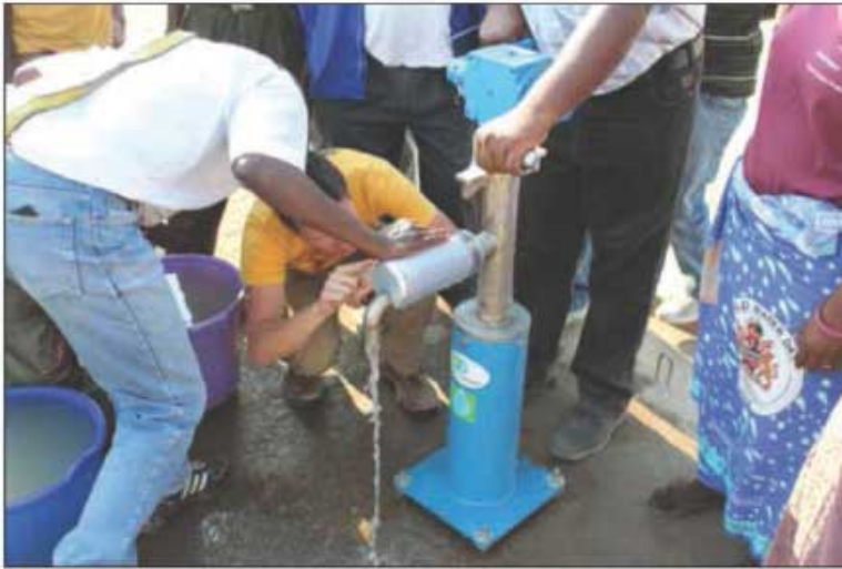
A LifePump in Malawi, Africa, is outfitted with a spout-mounted data logger, developed by SonSet Solutions (Elkhart, Ind.) to record usage information such as number of handle rotations and volume of water pumped. This information is useful for the multicountry Hundred Pump Project and water organizations interested in monitoring long-term pump performance. Photo provided by Design Outreach.
